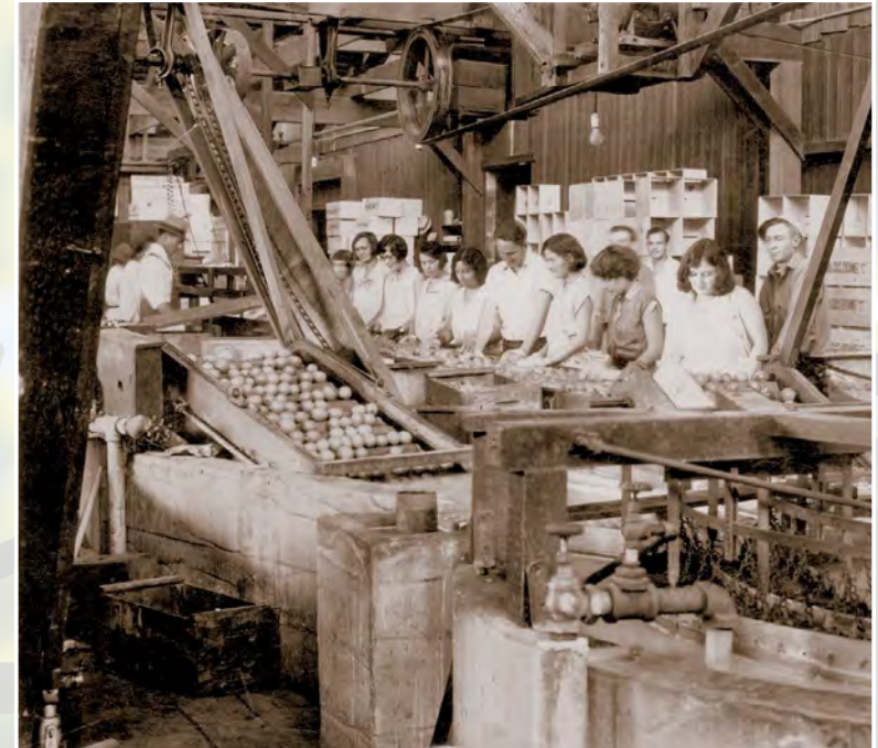
Chula Vista's lemon packing plants used assembly lines to wash, sort and box the fruit for shipping. Employees—like these pictured in the 1920s—did most of the work by hand.
