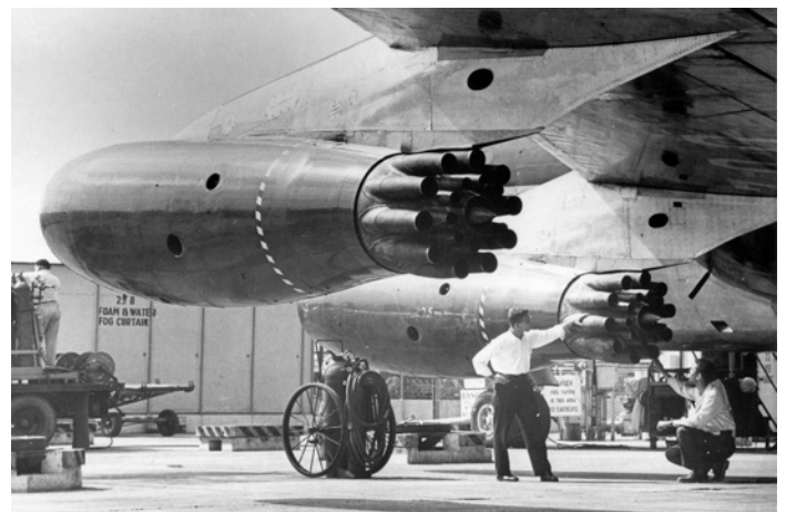
Rohr designed the exhaust with sound suppression for the Boeing 707.
